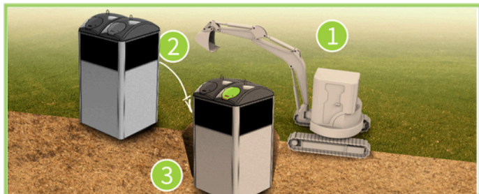
1. Dig a hole 2. Place the RBin in the hole 3. Fill the hole
